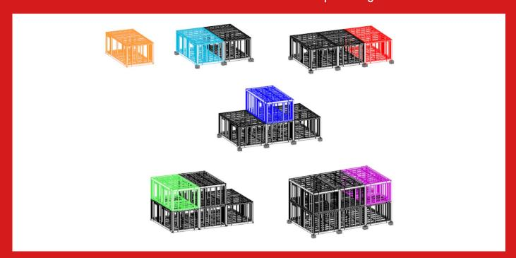
The pods contain rooms which were heavily M&E dependent and contained fixed furniture which need to be manufactured and finished at Hadley's Offsite facility.
